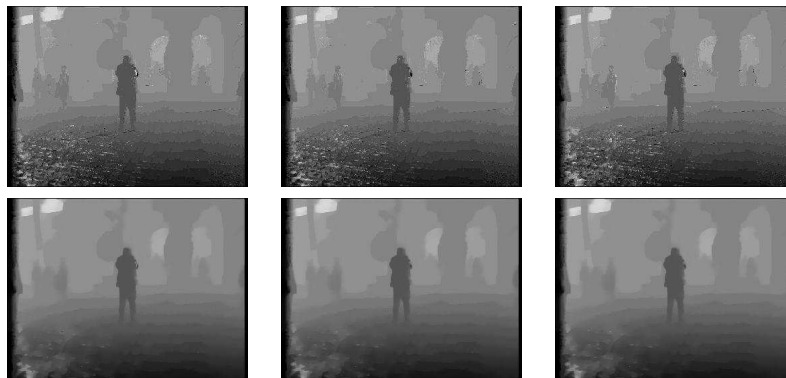
Figure 3: Example: Video disparity refinement. Top: Input. Bottom: Recovered. Time elapsed: 12.1 seconds for 10 frames.
