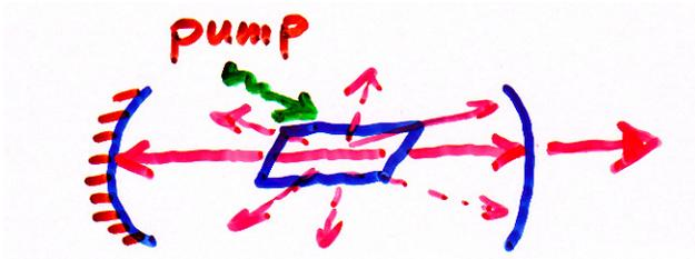
contained within a resonant cavity that provides feedback. Spontaneous emission from the active medium is reflected from the end mirrors and is reinforced by additional stimulated
