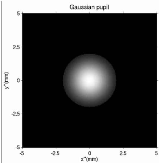
$$H(r'') = \text{circ}\left(\frac{r''}{R}\right) \times \exp\left(-\frac{r''^2}{2R_0^2}\right)$$
