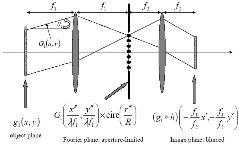
**In this case, image is blurred by the low-pass filtering effect of a finite aperture locating on the focal-plane.**
