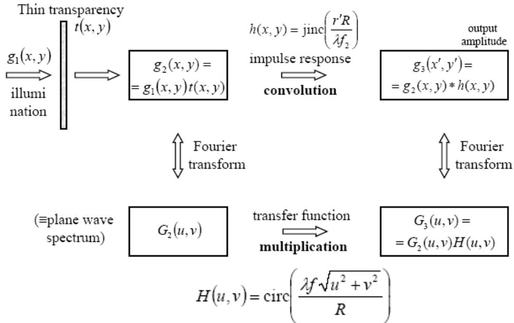
The transfer function of an 4f imaging system with a rectangular aperture in the Fourier plane:
