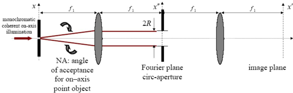
$$\text{jinc}\left(-2 \frac{R}{f_1} \frac{x'}{\lambda}, -2 \frac{R}{f_1} \frac{y'}{\lambda}\right) \equiv 2 \frac{J_1\left(2\pi \frac{R}{f_1} \frac{r'}{\lambda}\right)}{2\pi \frac{R}{f_1} \frac{r'}{\lambda}} = 2 \frac{J_1\left(2\pi(\text{NA})\frac{r'}{\lambda}\right)}{2\pi(\text{NA})\frac{r'}{\lambda}}$$
