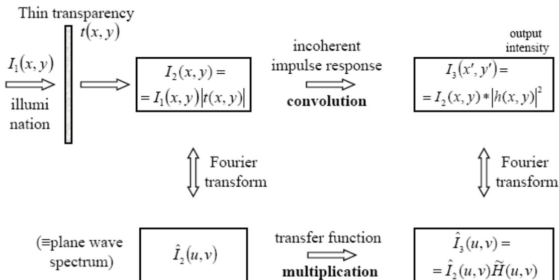
transfer function of incoherent system:  $\tilde{H}(s_x, s_y)$  **optical transfer function (OTF)**
