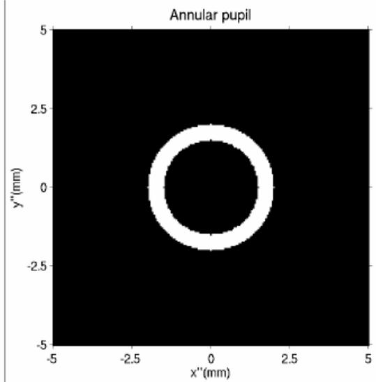
$$H(r'') = \text{circ}\left(\frac{r''}{R}\right) - \text{circ}\left(\frac{r''}{R_2}\right)$$
