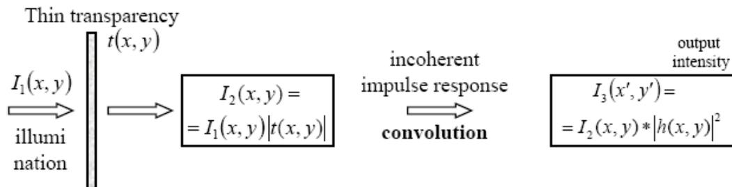
Incoherent imaging is *linear in intensity*
