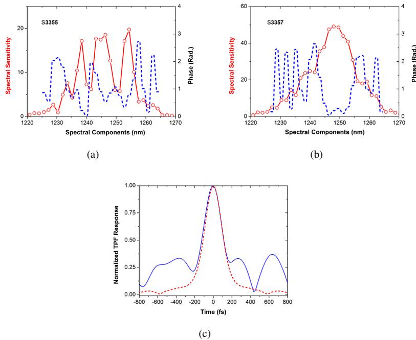
Fig. 6. Spectral-phase sensitivity curves of ccTPF and the spectral-phase patterns used to generate maximum ccTPF signal from the InAs quantum dot device with (a)  $\text{In}_{0.18}\text{Ga}_{0.82}\text{As}$ , (b)  $\text{In}_{0.18}\text{Ga}_{0.82}\text{As}_{0.8}\text{Sb}_{0.2}$  strain-reducing layer. (c) Fourier transform of the spectral-phase sensitivity profiles shown in (a) blue solid curve and (b) red dashed curve.
