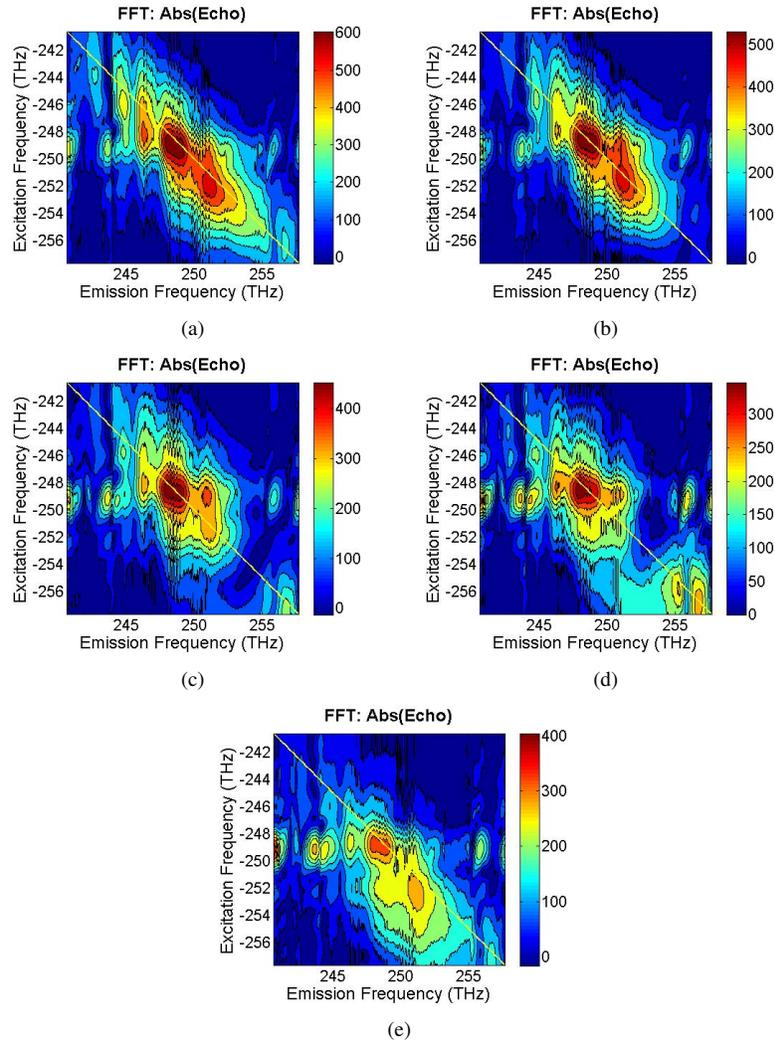
Fig. 7. 2D coherent spectroscopy of the InAs QDs device with an  $\text{In}_{0.18}\text{Ga}_{0.82}\text{As}$  strain-reducing layer. The device was excited by three ultrashort laser pulses with a spectrum covering from 1164 nm (258 THz) to 1246 nm (240 THz). During the 2D CS measurements, the waiting time was fixed at (a) 0 fs, (b) 33 fs, (c) 67 fs, (d) 100 fs, and (e) 234 fs. Note 249 THz=1029.8 meV=1203.4 nm, 251 THz=1038.1 meV=1194.4 nm, 252 THz=1042.2 meV=1189.7 nm, respectively
