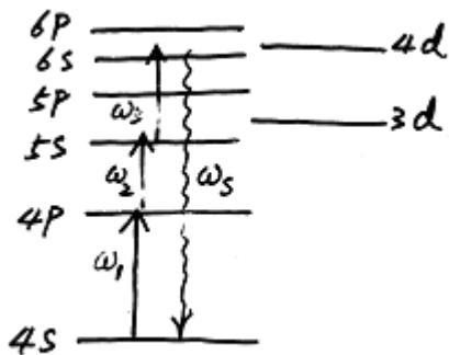
e.g., FWM for time-resolved infrared spectroscopy
