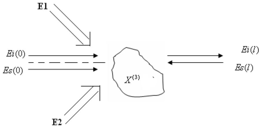
In this case, two pump beams are used instead of one field as in optical parametric amplification based on  $\chi^{(2)}$  effect.
