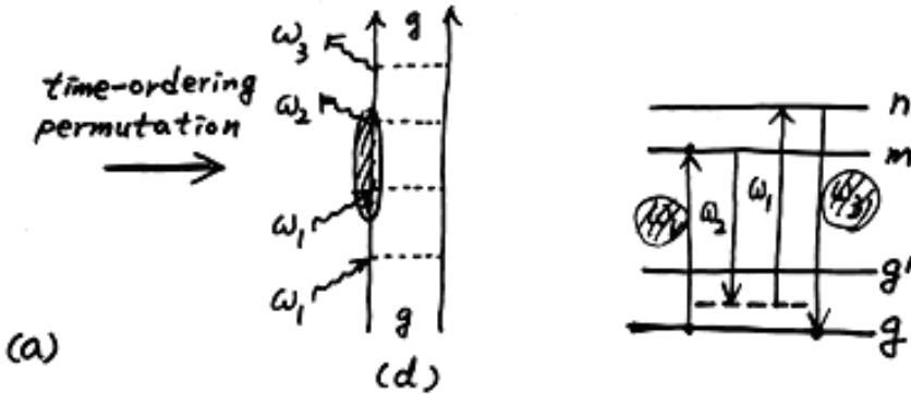
$$\chi_R^{(3)}(\omega_3)|_d = -\frac{Ne^4}{\hbar^3} \sum_m \rho_{gg}^{(0)} \left[ \frac{r_{gn}^i}{(2\omega_1 - \omega_2 - \omega_{ng} + i\Gamma_{ng})} \cdot \frac{r_{nm}^k r_{mn}^j}{(2\omega_1 - \omega_{mg})} \cdot \frac{r_{ng}^l}{\omega_1 - \omega_{ng} + i\Gamma_{ng}} \right]$$
