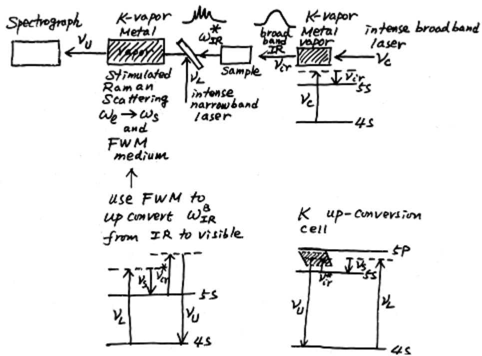
The conversion from IR to the visible is effectively uniform over a relatively wide spectral range. The up-converted signal thus provided a faithful reproduction of the spectral intensity.
