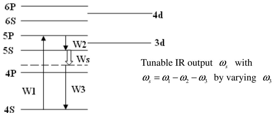
$$\chi_R^{(3)} \approx \frac{Ne^4}{\hbar^3} \sum_{sp} A_{sp} \underbrace{\langle 4s | r_j | 4p \rangle}_{\omega_2} \underbrace{\langle 4p | r_i | 5s \rangle}_{\omega_3} \underbrace{\langle 5s | r_k | 5p \rangle}_{\omega_1} \underbrace{\langle 5p | r_e | 4s \rangle}_{\omega_1}$$
