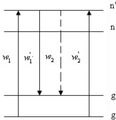
$$\chi_R^{(3)}(\omega_2 = \omega_2 - \omega_1 + \omega_1) \rightarrow \omega_2 \omega_1 \omega_1 \omega_2$$
