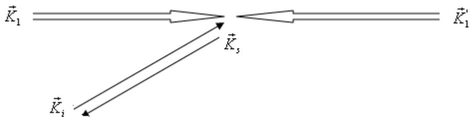
$$\begin{aligned} \rho_s^{(3)}(\vec{K}_s = -\vec{K}_i, \omega) &= \chi^{(3)}(\omega) : E(\vec{K}_1)E'(-\vec{K}_1)E_i^*(\vec{K}_i) \\ &= \underline{A}(E_1 \cdot E_i^*)E_1 + \underline{B}(E_1 \cdot E_i^*)E_1 + \underline{C}(E_1 \cdot E_1)E_i^* \end{aligned}$$
