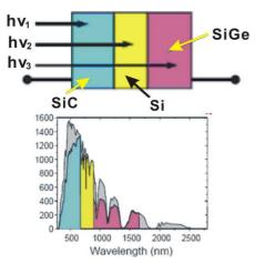
We shall improve the utilization efficiency of broadband solar photons in a PV device with a graded bandgap thin film system. This concept can be understood easily in the left diagram: If the heterostructure of a graded bandgap PV cell has a gradient of bandgap energy with reducing  $\boldsymbol{E}_g$  from the front surface, an additional voltage arises owing to separation of the electrons and
