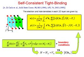
The self-consistent procedure can be implemented as depicted in the diagram on the left by integrating the TB procedure with Poisson equation to determine the built-in field that will be used to separate the photo-excited electrons from holes carriers.
